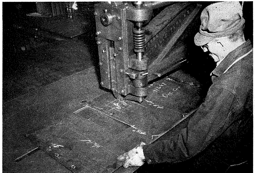
ORVILLE POTTS uses the nibbler to cut out holes in a section of a Special No. 35 Assembled Dust Collector. A section has been cut out just in front of his left hand. The nibbler is cutting the third side of an oblong cutout.
